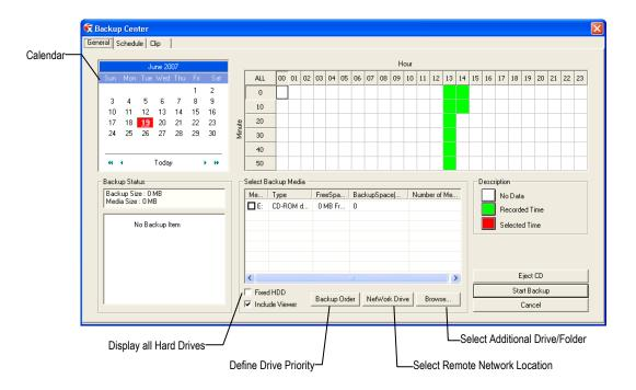
Hour / Minutes Recording data displays in hourly (24 horizontal columns) and 10 minute (6 vertical cells) segments.
