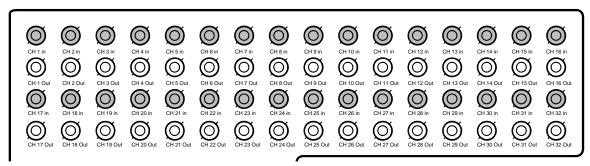
The video inputs are RG-59 BNC connectors. Plug one end into the video source (DVD, Camera, etc.) and plug the other end into the desired BNC input on the DVR unit.
